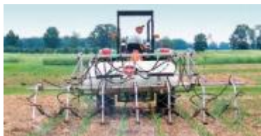
Flaming at the base of corn plants controls weeds within the row in an organic research plot at the W.K. Kellogg Biological Station, Hickory Corners, MI.
